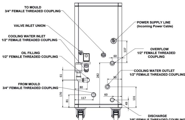
Thermotech Power oil mold temperature controllers with indirect cooling are used in various industries, particularly in injection molding, to maintain the optimal temperature of molds during production processes.
